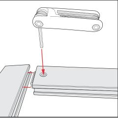
Extrusion & Lock Connection
