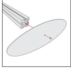
Base Plate & Extrusion Connection
